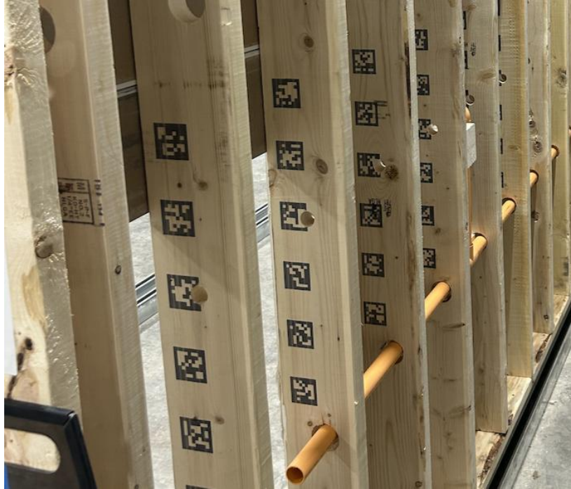
Figure 14: Wall studs preprinted with alignment lines and QR codes ready for assembly at Reframe’s pilot microfactory. Source: Authors, photograph taken 2025.
