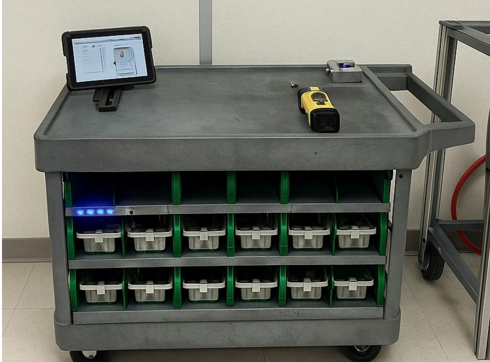
Figure 13: Pick to light cart with tablet-based work instructions at Reframe’s pilot microfactory. Source: Authors, photograph taken 2025.
