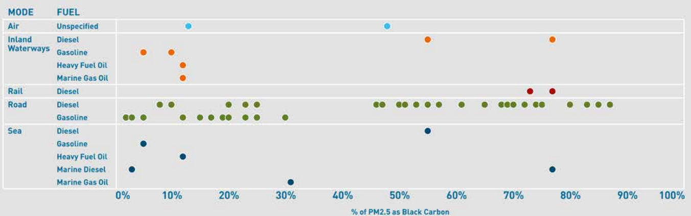
Figure 6 Examples of different PM2.5 to black carbon speciation factors for different modes, vehicle types and fuels. Each point represents a different study and/or vehicle type. A table of speciation factors is available in Appendix 4.
