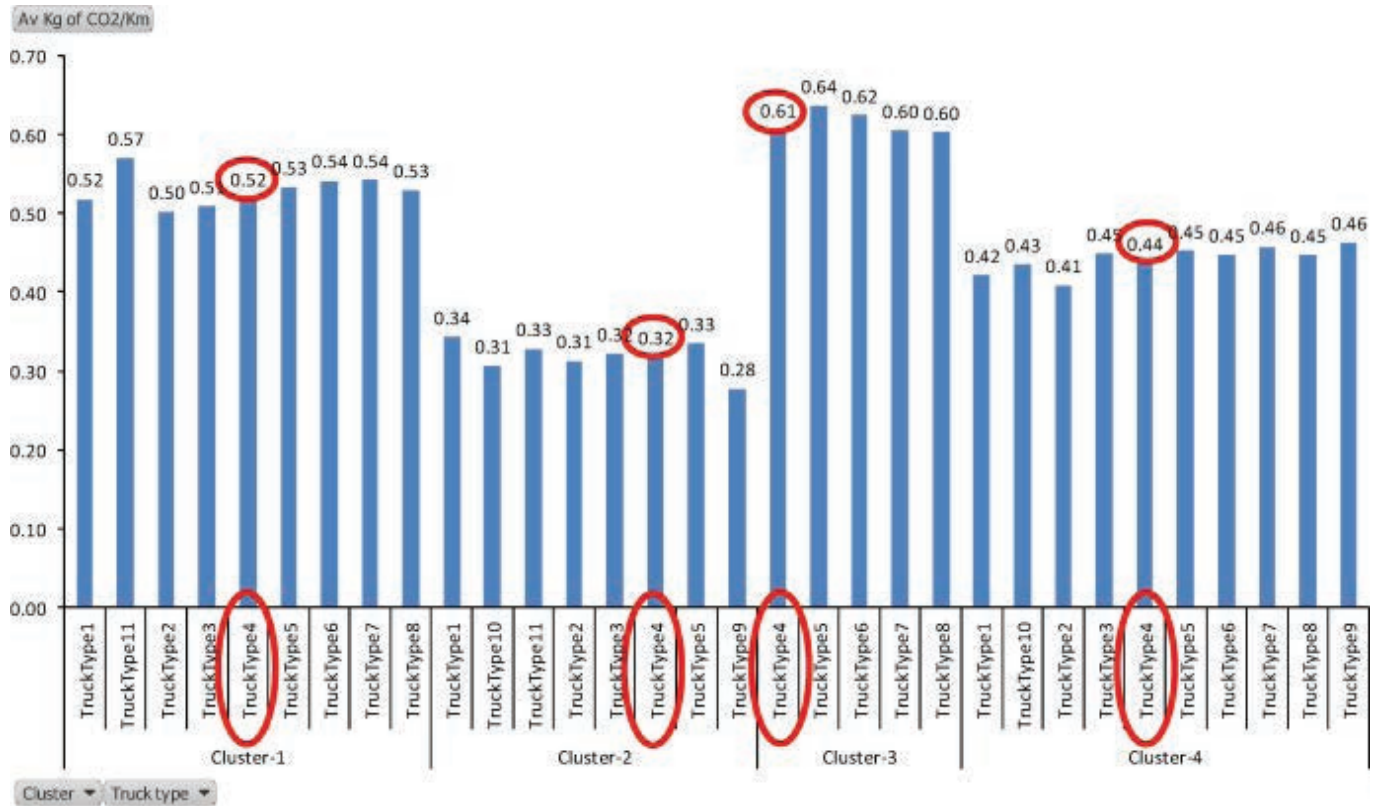
Figure 2. Average emission factors per type of truck per cluster. (Source: Velázquez-Martínez et. al., 2016)
